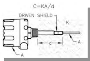
The driven shield section of the probe enables the electronic circuitry to ignore product build-up on the probe that would otherwise cause false sensing. The driven shield is activated with the same radio frequency potential as the sensing probe. Since current cannot flow between identical potentials, the driven shield blocks current flow from the active probe to the vessel wall through the material build-up, thereby eliminating the sensing of the material build-up.
