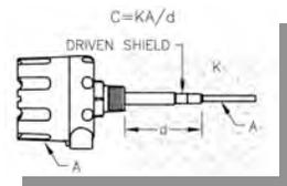
The sensor's active probe and the vessel's wall makeup the two plates (A = area) of a capacitor which are separated by a fixed distance (d). The probe's insulator and surrounding air provide the dielectric material (with dielectric constant "K"). As the air (K = 1.0) is displaced with any other material (K > 1.0), the capacitance effect (C) is enhanced, thereby changing the application's impedance.
