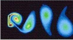
A practical consequence of the regular, periodic flow is that the forces on the body are also periodic. Because the flow is asymmetric fore and aft as well as in the direction transverse to the flow the body will experience both an oscillating drag and lift. If the frequency of the **shedding** is close to a structural frequency, resonance can occur, usually with unpleasant results.
