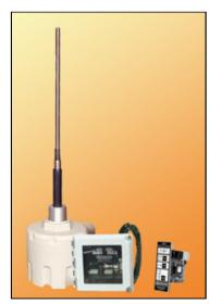
Monitor's TrueCap® Model MK-2 RF capacitance point level sensor is designed to provide a superior and stable sensitivity threshold making it suitable for a variety of powder and bulk solids, liquid and slurry applications. The **available split architecture design** is ideal for applications involving high temperature or vibration. The probe and electronics are housed in separate enclosures that are mounted apart for each other. This design removes the electronics from the tough conditions.
