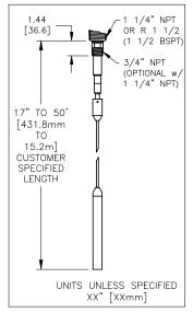
\*Unit with 1-1/2" BSPT connection is provided with M20 cable glands.
